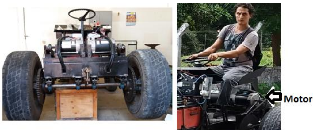
Figure 109 – Motors on top of the rear axle below the driver's seat
