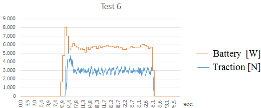
Figure 121 – Drawbar force and battery power during Test 6
