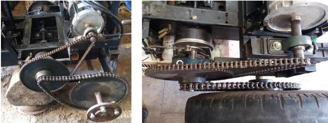
Figure 110 – Two stage chain drive (guards removed)
