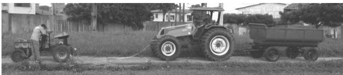
Figure 118 –Test train with prototype electric tractor dragging a Valtra A Series tractor and a two axle trailer as its load
