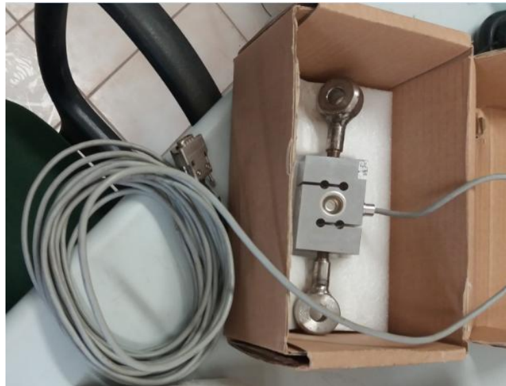
Figure 69 – Load cell, Model: HBM, RSCC
