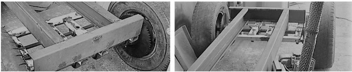
Figure 107 – Rear axle with support structure mounted to the main chassis
