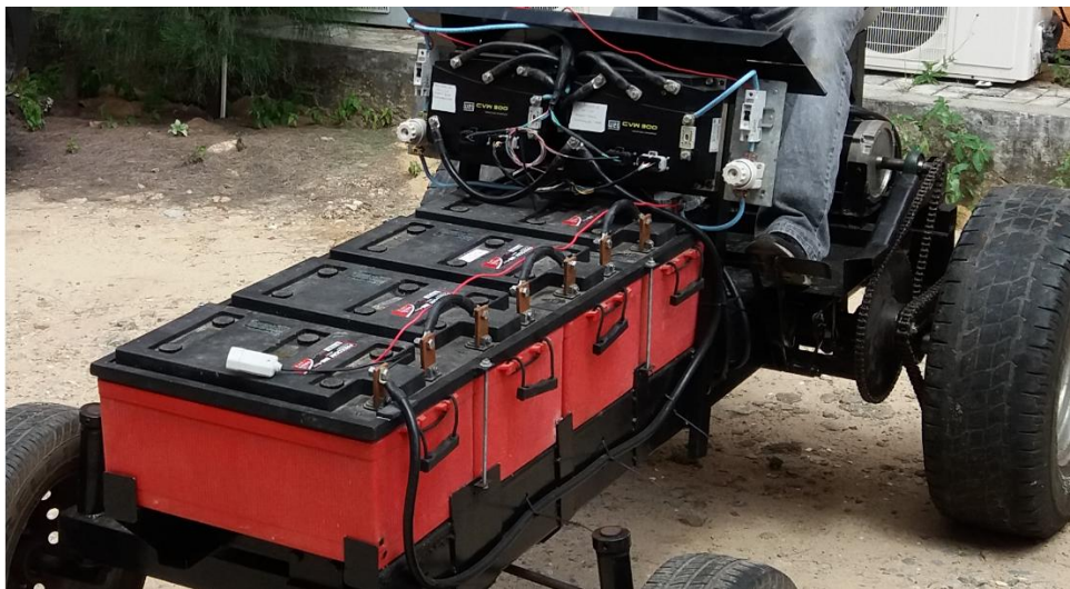
Figure 112 – Battery packs at the front of prototype electric tractor
