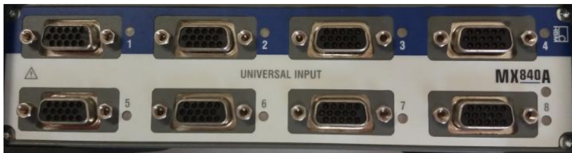
Figure 70 – Data logger, HBM Quantum X MX804A
