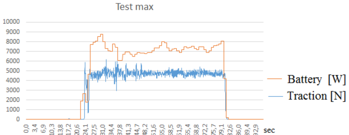
Figure 122 – Drawbar force and battery power during test “max”
