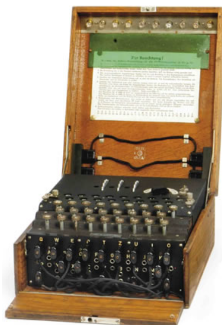
Figure 1.1: Enigma rotor-machine used in world war II by the Nazi German army.
