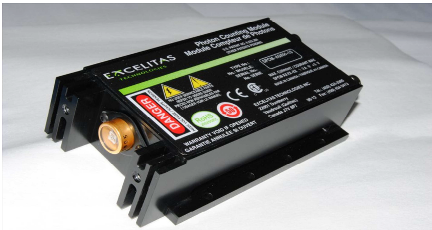
Figure 5.4: SPCM module from Excelitas, model SPCM-AQRH with an encapsulated Si-APD attached.
