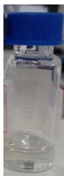
Figura 5- Clean-up contendo 150 mg MgSO 4 , 25mg PSA e 10 mg de GCB.
