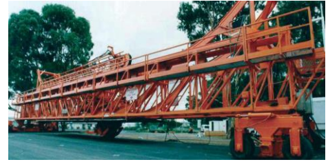
(c) Accelerated Loading Facility (Virgínia)
