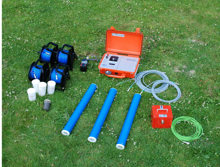
Figure 45: MT equipment for data acquisition. Three magnetometers (blue), electrodes (white) and ADU acquisition system (orange box).
