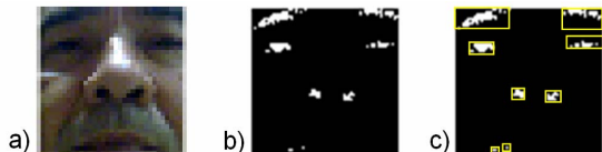
Figure 6. Result of feature segmentation, followed by point clustering using t=0.96 , k=5 , n_c=8 .
