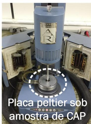
**Figura 22:** Amostra de CAP submetida ao *frequency sweep* no DSR AR-2000
