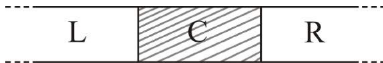
Figure 15: Simplified model, for a system formed by two contacts (L and R) separated by a conductor (C).
