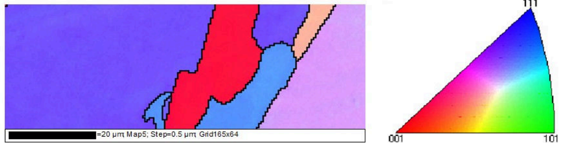
Figure 34 - Selected region and the orientation map for the EBSD measurement of the AL-6XN PLUS™ steel heat treated at 600 °C for 960 h.
