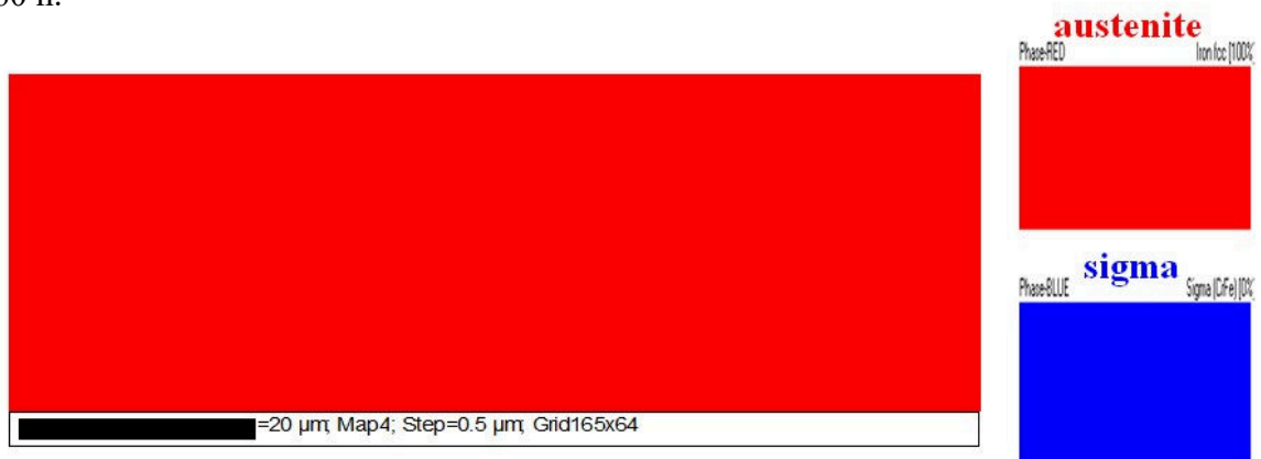
Figure 35 - EBSD map of the phases for the AL-6XN PLUS™ steel heat treated at 600 °C for 960 h.
