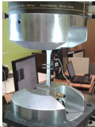
Figure 3.11. Use of extensometer to measure the stiffness modification during load/unload tensile testing.
