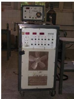
Figura 39. Fonte Inversal 300 – LABSOLDA/UFSC.
