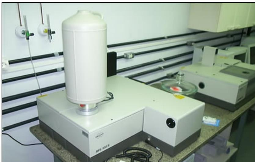
FIGURA 5.1 – Espectrômetro FT-Raman<sup>59</sup>.
