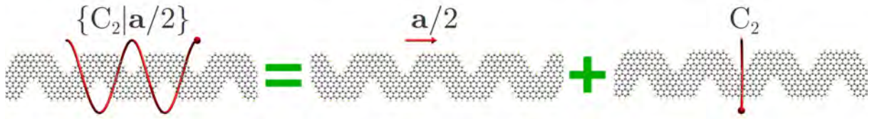
Figure 8.4: Improper rotation symmetry for the GNW's unit cell.
