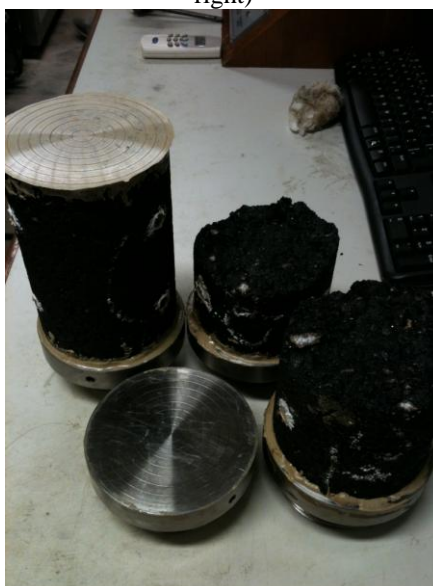
Figure B1 – Unsticking of the glue from the endplate (sample at the left) and failure in the mixture (sample at the right)
