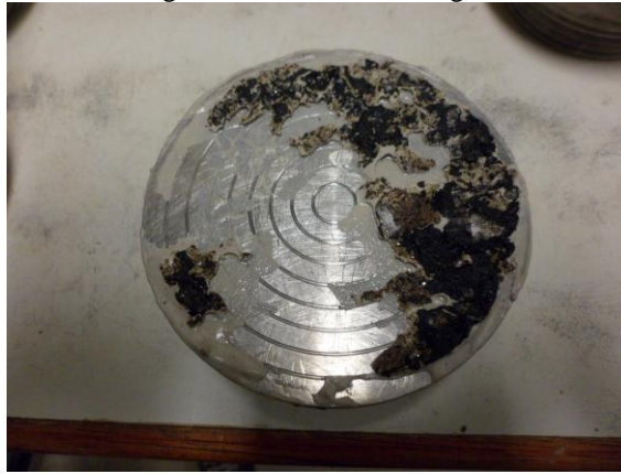
Figure B2 – Failure in the glue
