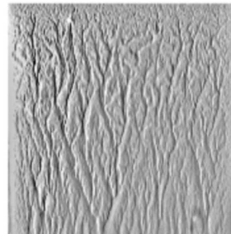
FIG. 1. Pattern observed in erosion experiment with commercial abrasive powder. Angles between 30^\circ and 90^\circ were found for different chevron alignments [14].
