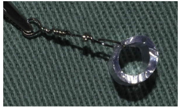
FIGURE 2. The other end of the orthodontic stainless steel wire is inserted through the hole in the tube, pulled back, and twisted.
