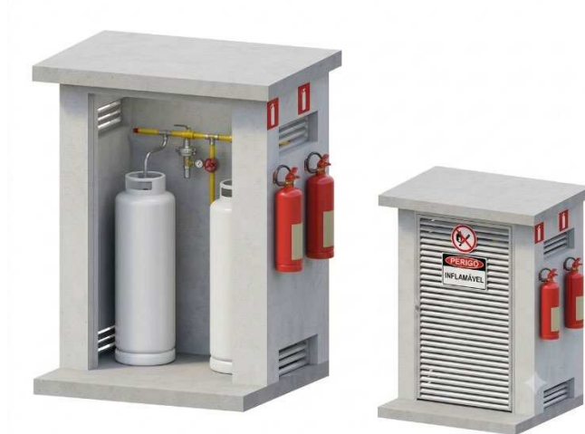
Figura 17: Central de GLP
