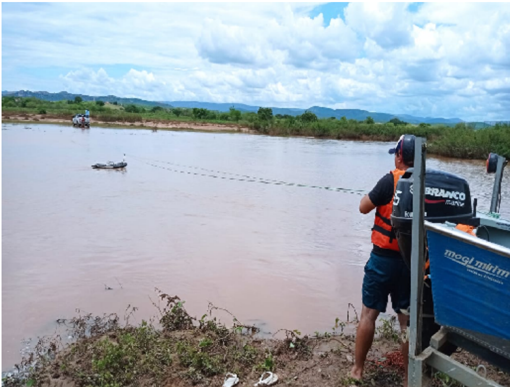
Figure S2.1 - River discharge measurement using RiverSurveyor M9 ADCP in the stream gauge.
