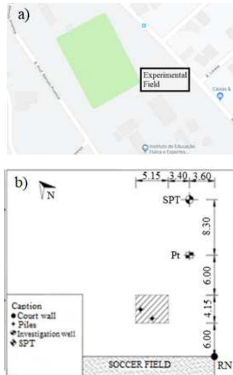
Figure 2 (a) Site map of study, and (b) Overview and points of sample collection and standards penetration tests
