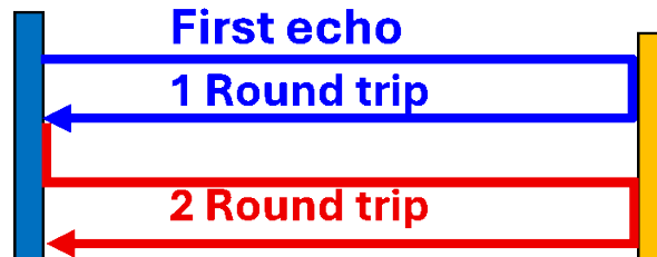
Figure 6 – Diagram illustrating the first two acoustic echoes generated by multiple round trips of the wave between the transducers. The first echo corresponds to one complete trip (1 round trip) and the second echo to two complete trips (2 round trips), allowing precise measurement of the wave's transit time by the interval between consecutive echoes. (Created by the author, 2025)
