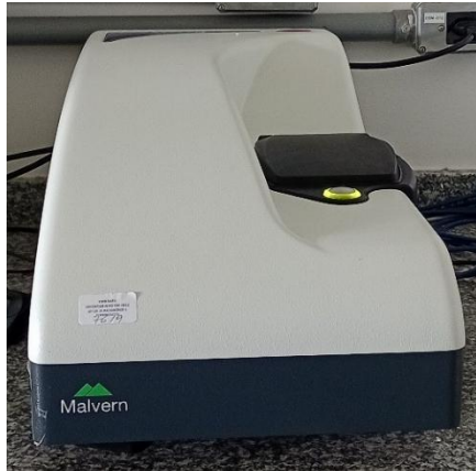
Figura 14 – Zetasizer Nano ZS
