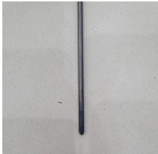
Figure 49 – Electrode tip after four passes of TIG welding using 216 A current.
