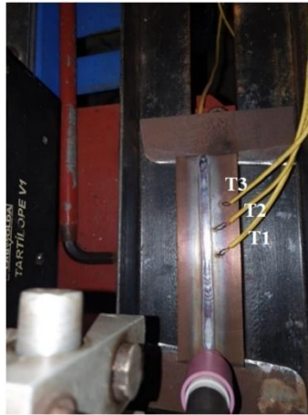
Figure 44 – Sample of AISI 409 steel after fourth TIG welding pass with 165A current.
