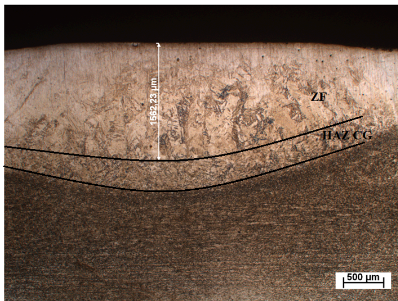
Figure 52 – Microstructures of AISI 409 steel after first welding pass with an average current of 216A.
