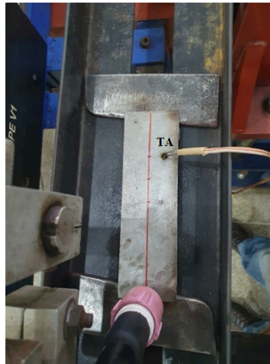
Figure 46 – Top of AISI 409 steel sample with a thermocouple fixed 13 mm from the center of the weld bead.
