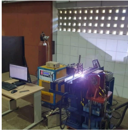
Figure 45 – Workbench in operation carrying out TIG welding process.
