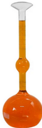
Figure 31: Determination of the actual specific mass of the ash using Le Chatelier's flask.
