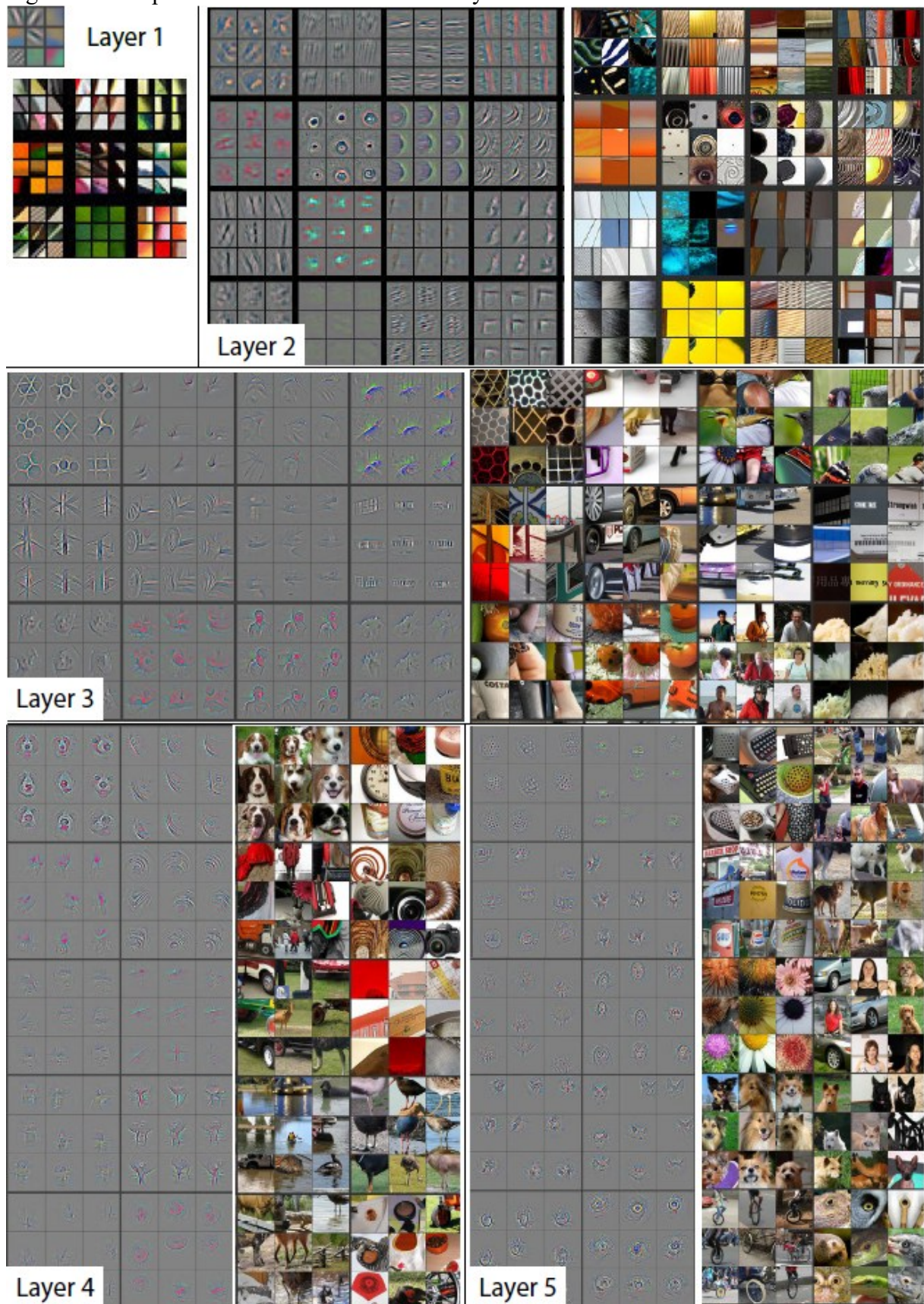
Figure 18 – Representation from the first five layers of a CNN
