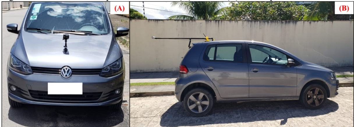
Figure 4 – Vehicle cameras placements – front (A) and rear (B) camera positions
