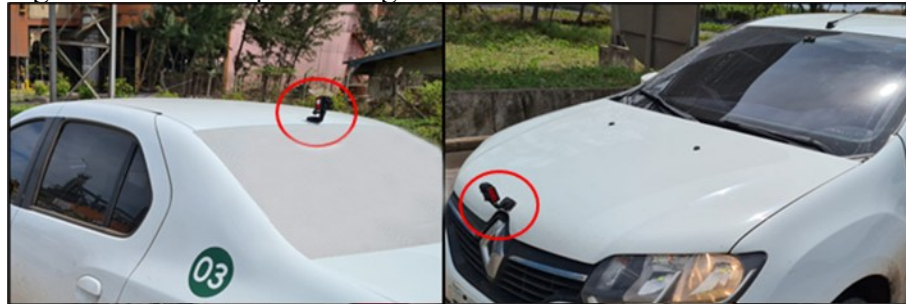
Figure 6 – Camera positioning in the vehicle
