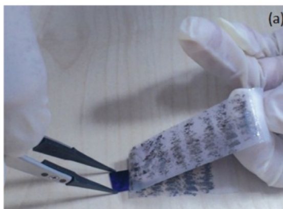
Figure 9 – Cleaving the bulk graphite using the Scotch tape.
