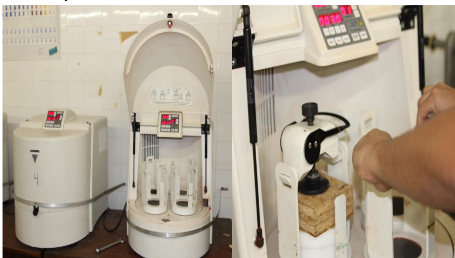
Figure 22 – Planetary ball mill.
