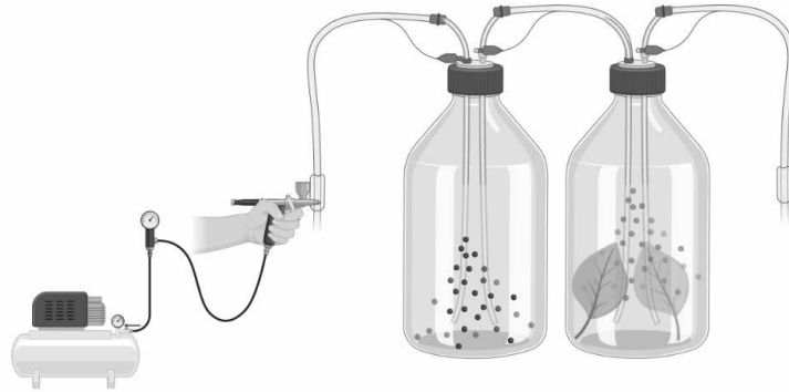
Figure 42 – Exposure of particles to leaves at a laboratory scale
