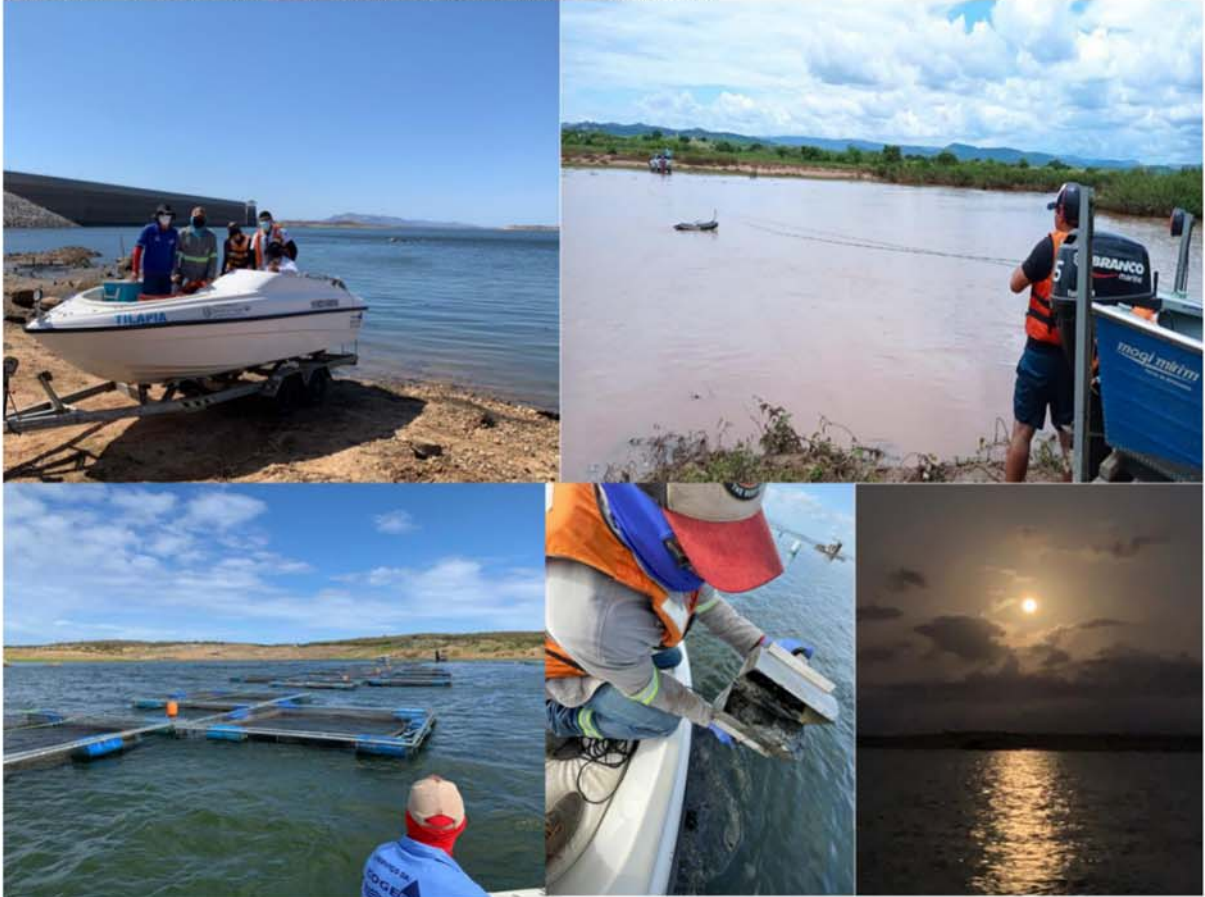
Figure S 66 - Water quality monitoring campaigns with river flowrate measurements, reservoir's bed sediment sampling, and water sampling.
