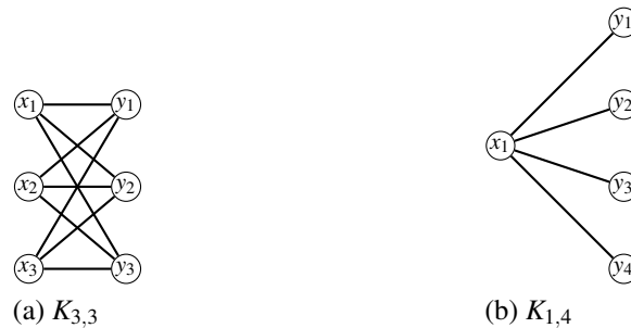
Figure 3 – Two complete bipartite graphs: (a) K_{3,3} and (b) K_{1,4} , the star of order 5.
