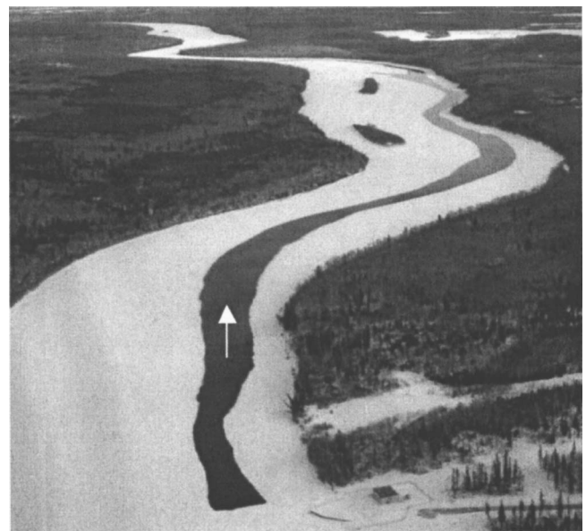
Fig. 3. Open-water lead in the Athabasca River downstream of Al-Pac diffuser, with indication of flow direction
