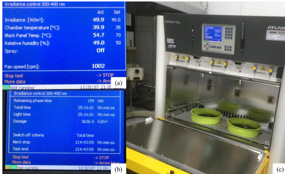
Figure 8 – Weathering chamber used for UV induced aging
