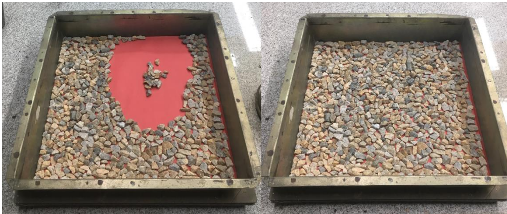
Figure 44 - Determination of rate of aggregate using tray
