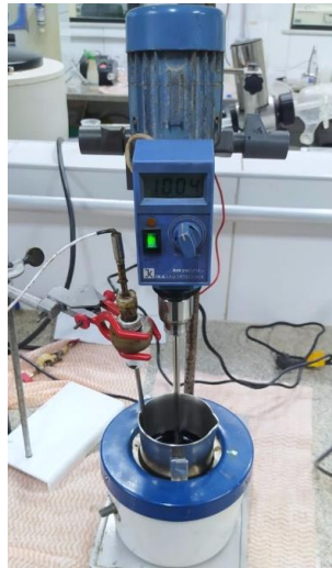
Figure 15 – Anti-stripping amine-based agent and binder mixing process.
