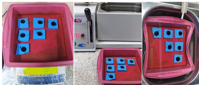
Figure 20 – Moisture conditioning of binders.
