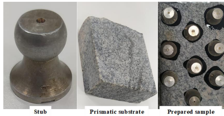
Figure 24 – Metallic stubs, prismatic substrate and sample ready for testing.
