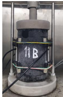
Figure 30 – Dynamic modulus test instrumentation.
