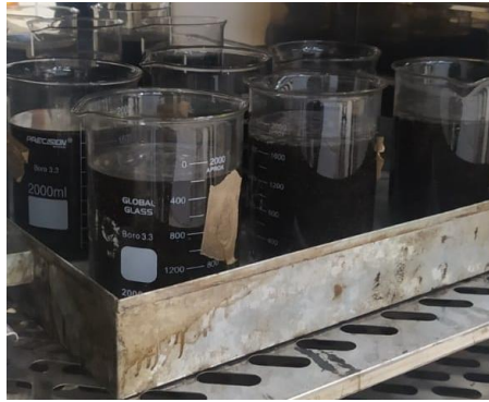
Figure 28– Water bath at 60^\circ\text{C} inside an oven.
