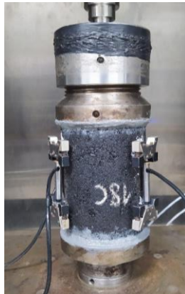
Figure 32 – Fatigue specimen instrumented at UTM-25.
