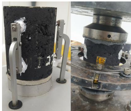
Figure 31 – Glued pieces and endplates.
