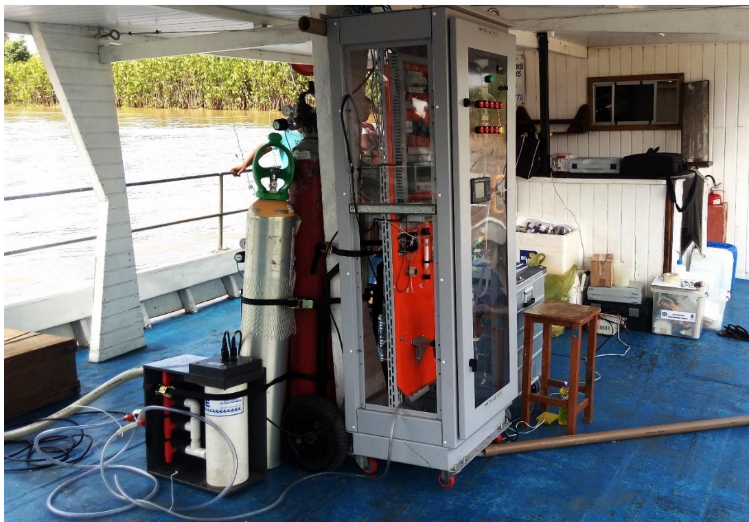
Figure 7. Equipment for the continuous and real time measurement of p\text{CO}_2 during the field work.
