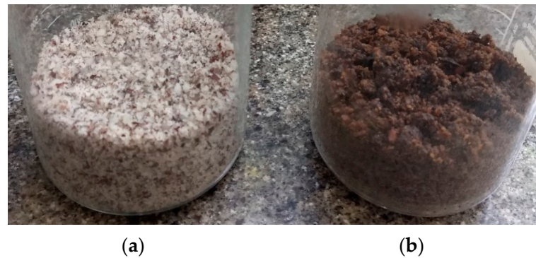
Figure 4. Fresh sample of ground babassu kernel (a). Aged sample of ground babassu kernel (b).
