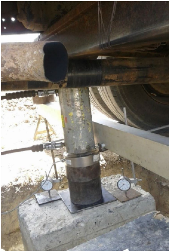
Fig. 7 Load being applied on a cap in CEGEF-UFC (Bonan 2017)
