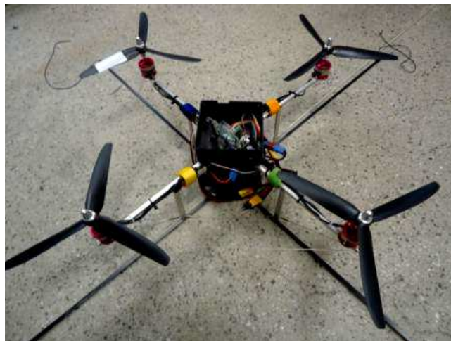
Figure 1. A picture of the developed UAV-type quadrotor.
