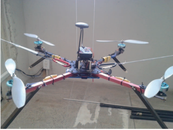
Fig. 1: Home-mounted quadrotor based on open technology.
