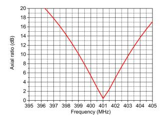
Fig. 4. Axial ratio as a function of the frequency for the standard antenna, in  $\theta=\phi=0\,^\circ.$
