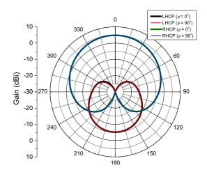
Fig. 23. Gain for the antenna with metallic fence with length of 10 cm.
