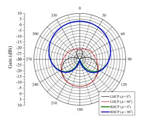
Fig. 12. Gain pattern for the antenna with two 8-cm cylindrical rods attached to each GND edge.
