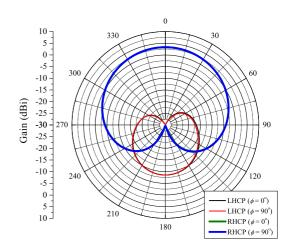
Fig. 13. Gain pattern for the antenna with four 8-cm cylindrical rods attached to each GND edge.
