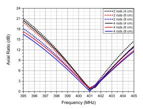
Fig. 11. Axial ratio as a function of the frequency for all cases employing cylindrical rods.
