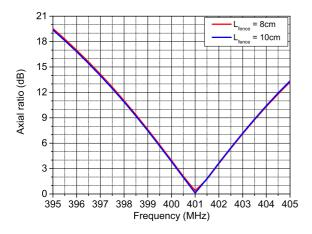
Fig. 21. Axial ratio as a function of the frequency for the metallic fence model, for  $\theta = \phi = 0^{\circ}$ .
