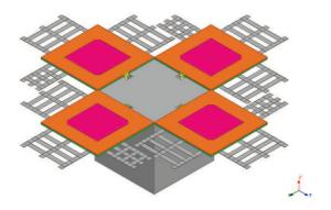
Fig. 24. Antenna array with metallic fences installed onto the nano-satellite.
