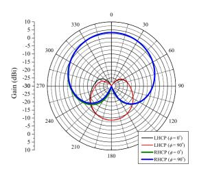
Fig. 18. Gain for the antenna with four metallic strips and length of 8 cm.
