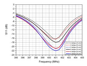
Fig. 15. Reflection coefficient as a function of the frequency for all cases of the metallic strips.
