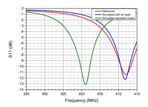
Fig. 8. Comparison between measured and computed results.
