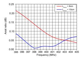
Fig. 28. Axial ratio as a function of the frequency for the antenna array with metallic fence model.
