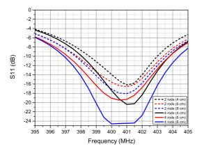
Fig. 10. Reflection coefficient as a function of the frequency for all cases employing cylindrical rods.
