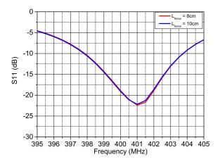
Fig. 20. Reflection coefficient as a function of the frequency for the metallic fence model.
