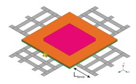
Fig. 19. Antenna structure using metallic fence.
