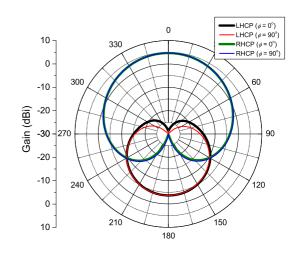
Fig. 22. Gain for the antenna with metallic fence with length of 8 cm.
