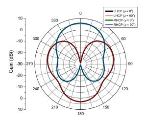
Fig. 25. Gain pattern for the antenna array with metallic fences and length of 8 cm.
