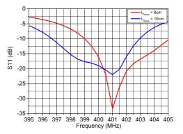
Fig. 27. Active reflection coefficient as a function of the frequency for the antenna array with metallic fence model.
