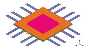
Fig. 14. Designed antenna with metallic strips.
