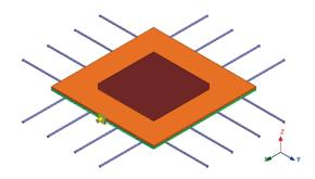
Fig. 9. Designed antenna with cylindrical rods.
