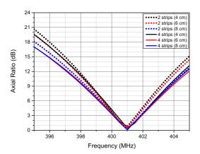
Fig. 16. Axial ratio as a function of the frequency for all cases of the metallic strips.
