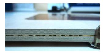
Fig. 7. Cross-sectional view of the prototype standard antenna.
