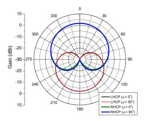
Fig. 5. Gain pattern for the standard antenna.
