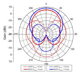
Fig. 29. Gain for the antenna array with metallic fences considering  $L_{fence} = 8$  cm and  $L_{fence} = 10$  cm.
