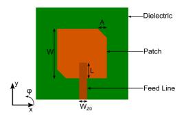
Fig. 3. Schematic top view of the designed antenna.
