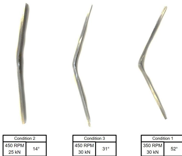
Figure 9.2 – Conditions of dissimilar butt joints of AISI 444/316L steels, produced by the FSW process, submitted to bending test.
