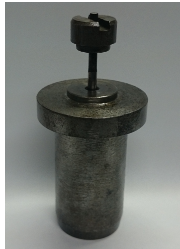
Figure 3. The piston-cylinder assembly.
