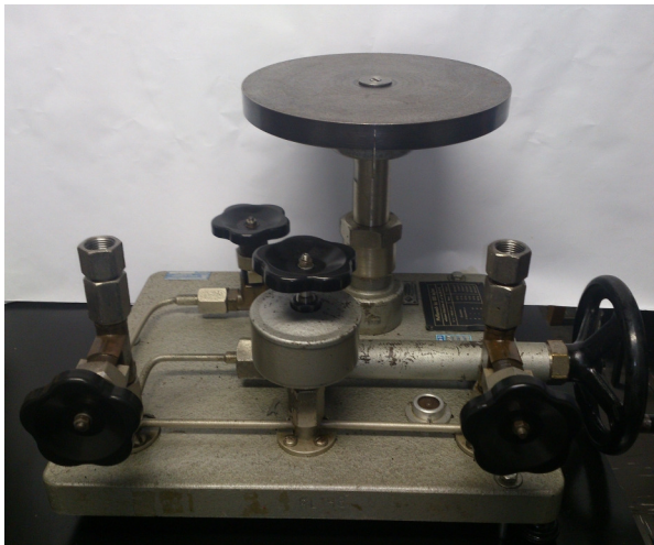
Figure 2. The VEB Gertewerk pressure balance studied.
