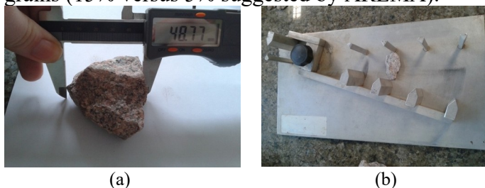
Figure 1 – Equipment for traditional characterization of form: (a) ABNT NBR 5564 (2011) e (b) ASTM D4791 (2010).
