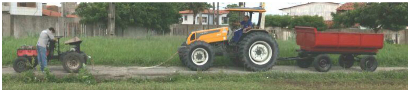
Fig. 8 Preparation for the test sessions: the dragged load, in this case, is composed of a two-axle trailer coupled to an ICE tractor model Valtra Series A
