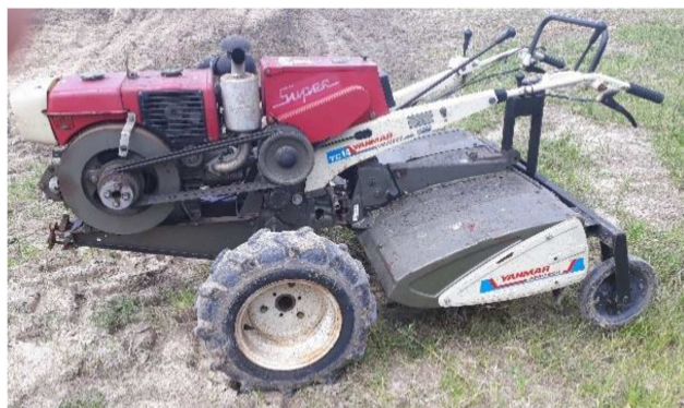
Fig. 18 10.3 kW ICE tractor manufactured by Yanmar Agritech
