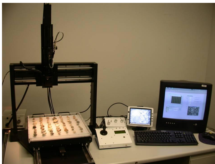
Figura 2: Aggregate Imaging System (AIMS)
