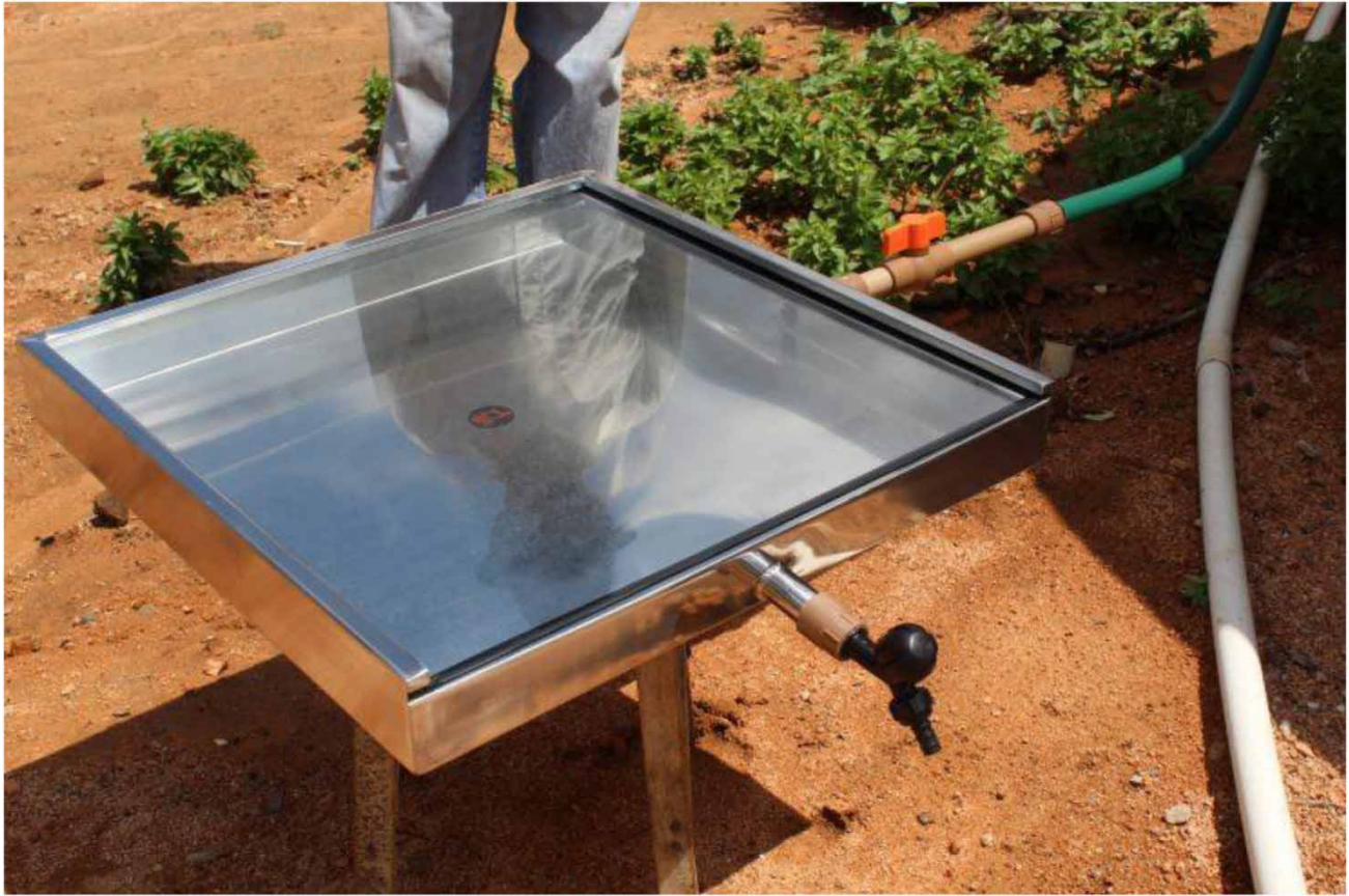
Figure 2 | Aqualuz unit used for removal of EC from cistern water using SODIS. External dimensions of 57 cm × 5 cm × 8 cm 3 (water depth of 5 cm).
