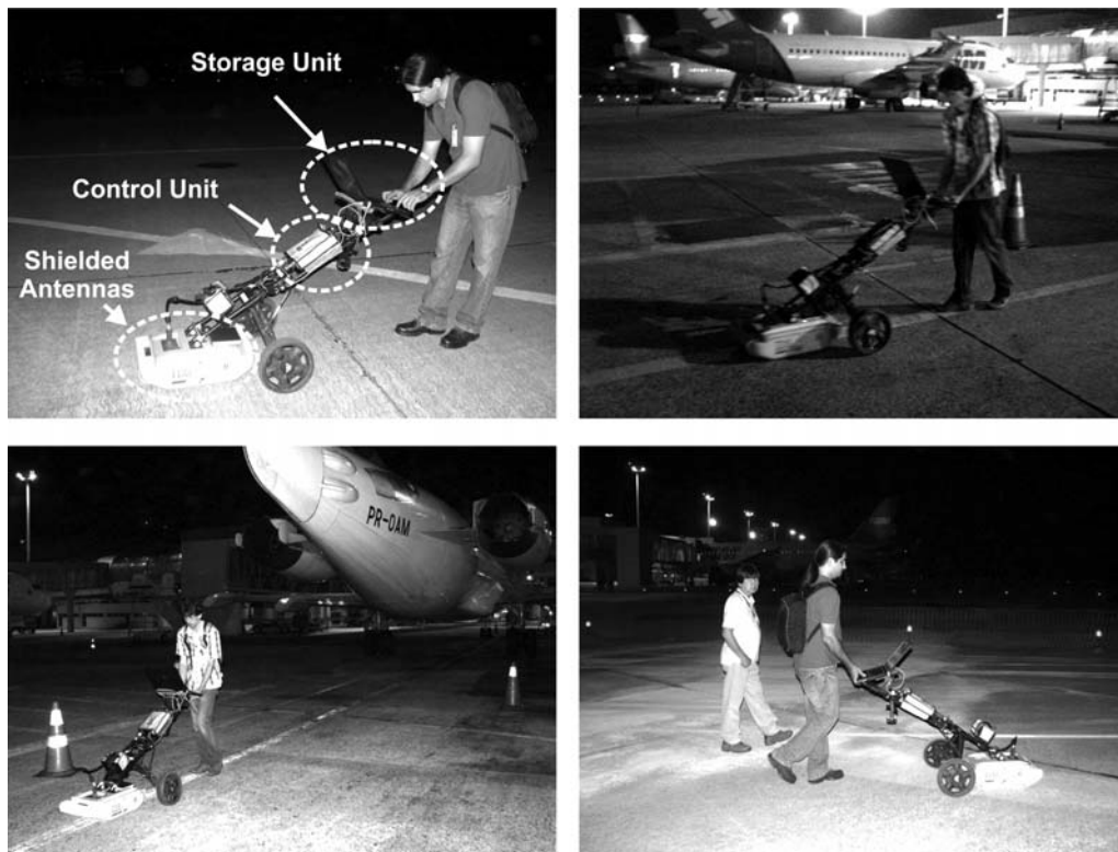
Figure 3 – Photos show the GPR data acquisition in part of the Santos Dumont Airport, Rio de Janeiro/RJ.
