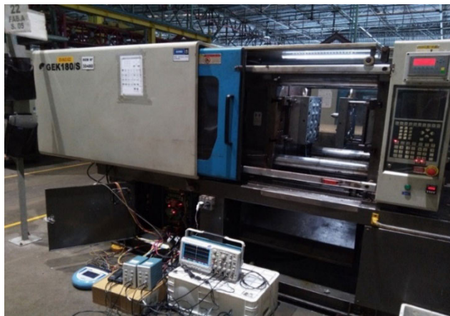
FIGURE 7. Measurement instruments associated with the plastic injection molding machine in a footwear factory.
