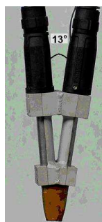
Figure 2. Angle of 13 degrees between the guns.
