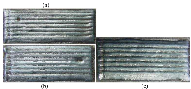
Figure 9. Photos of the layers deposited at a mean current of 120 A/wire: a) l_t > t_p ; b) l_t = 0 ; c) at random.
