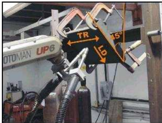
Figure 5. Position and direction of the gun displacement during the overhead trials.
