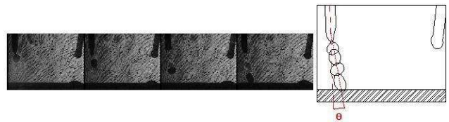
Figure 7. Deviation angle of droplet \theta = 6^\circ : the left electrode pulse current at the moment of the droplet detaching is of 280 A and of the right electrode is of 50 A ( I_m = 80 A and t_l = 10,2 ms).
