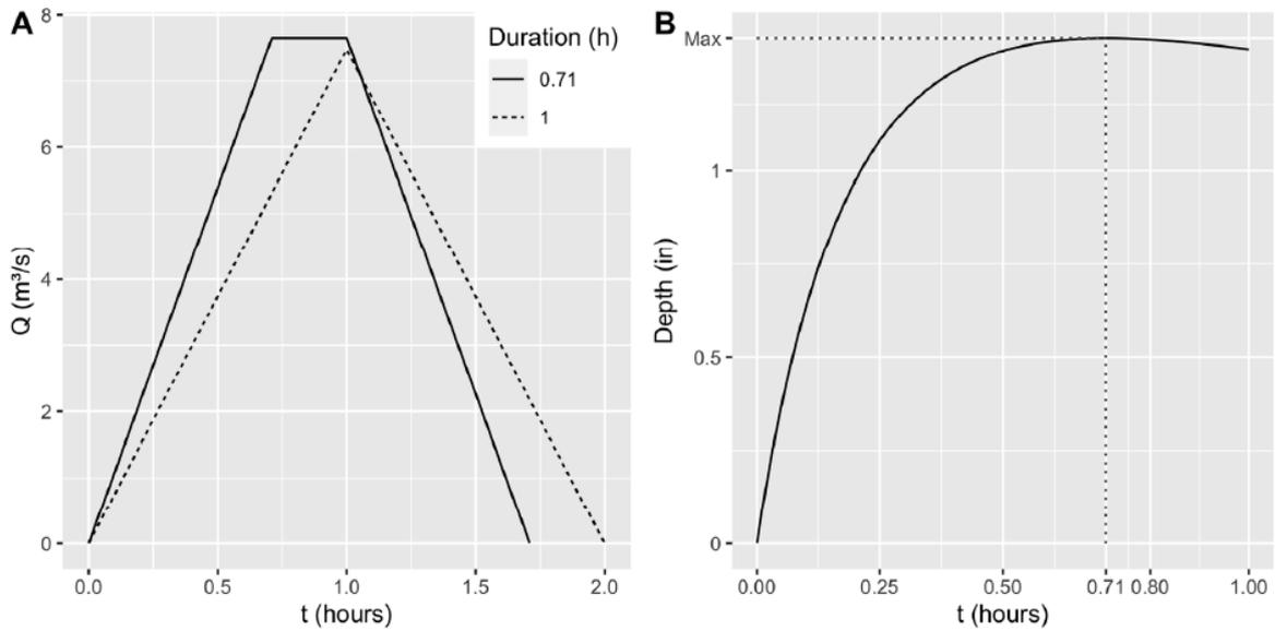
**Figure 1.** (A) Hydrographs resulting from the application of the South Bend ID with the Rational Method for rainfall durations  $t_d = 0.71$  h and  $t_d = 1$  h and  $t_c = 1$  h. (B) Depth Duration (DD) graph of the South Bend ID equation. In both graphs, the ID equation is for  $T_r = 10$  years.
