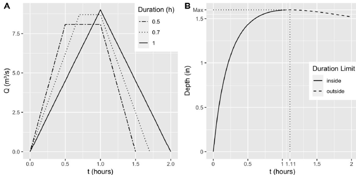
**Figure 3.** (A) Hydrographs resulting from the application of the Fort Wayne ID with the Rational Method for rainfall durations  $t_d$  equal to and 0.5, 0.7 and 1 h and  $t_c = 1$  h. (B) Depth Duration (DD) graph of the Fort Wayne ID equation. In both graphs, the ID equation is for  $T_r = 10$  years.
