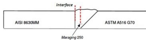
Figure 4. Charpy-V notch location in the front face of welded joint.
