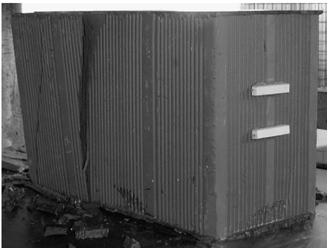
Fig. 10. Single block failure under compression. Failure occurred according to a vertical plane through the separation of “layers”.
